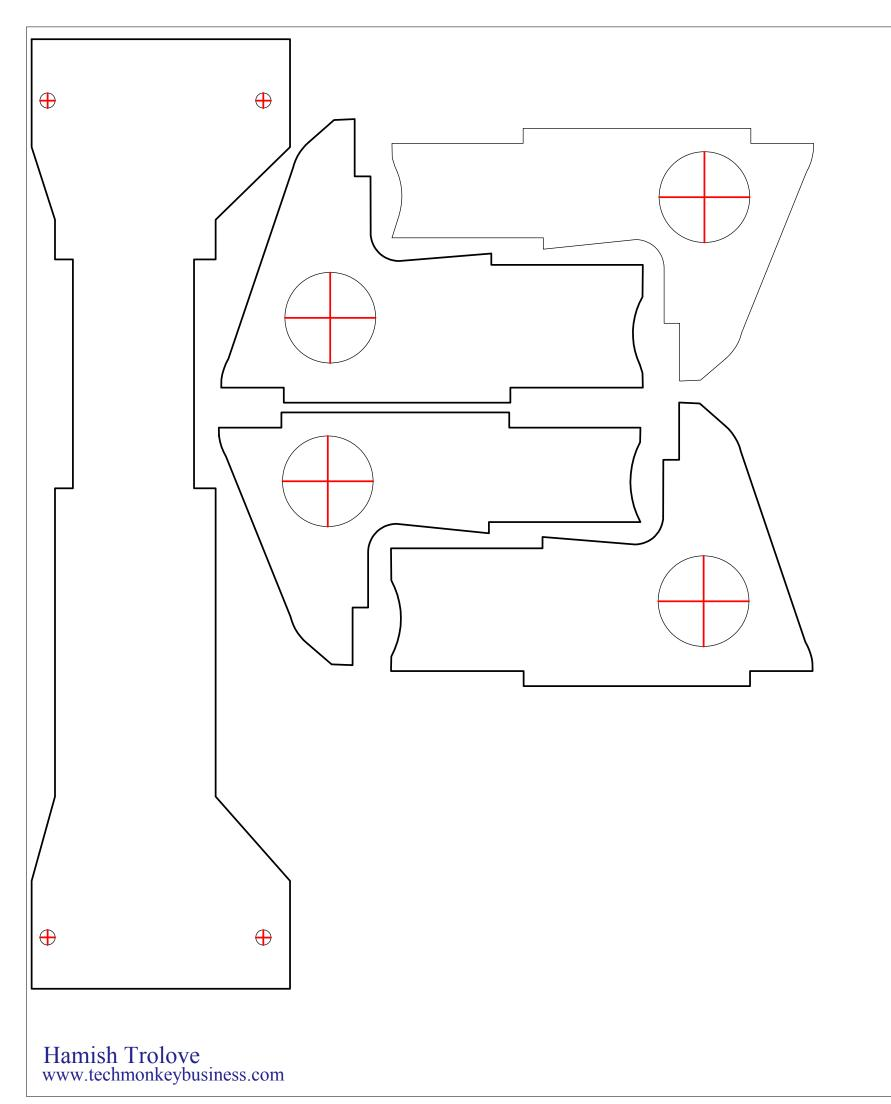
ROV Exterior Panels - V9 Material: 4 or 5mm Thick Acrylic Scale 1:1 When Printed Unscaled on A3
