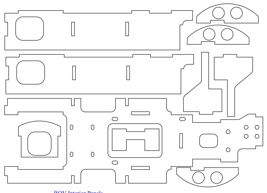
ROV Interior Panels Material: 3mm Thick Acrylic Scale 1:1 When Printed Unscaled on A3
