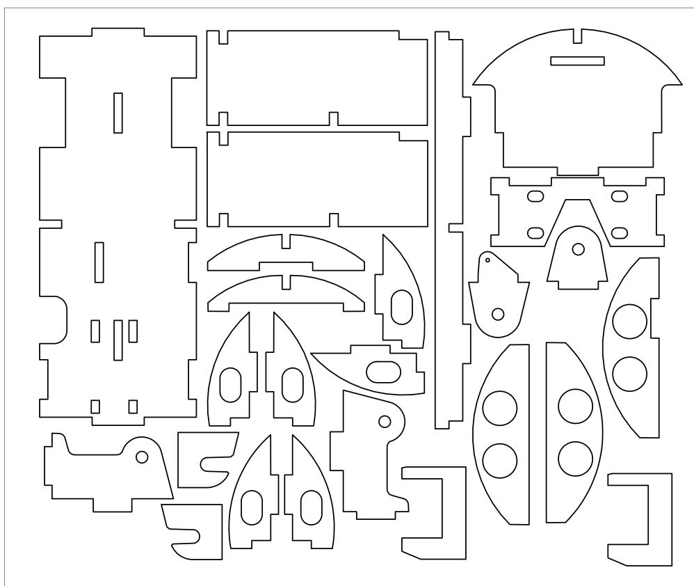
ROV Interior Panels Material: 3mm Thick Acrylic Scale 1:1 When Printed Unscaled on A3
