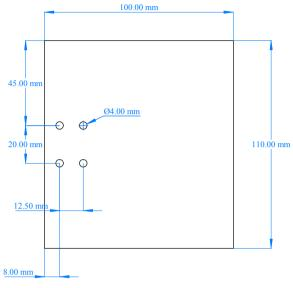
Camera Traveller Base Plate Drill to suit camera support
