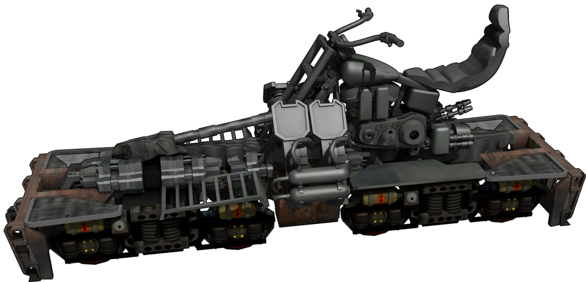
Illustration 3: The articulated rail bike concept.
