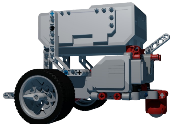
Two drive wheels and a caster wheel. Manoeuvrable and able to tolerate ramps and roughish surfaces.
