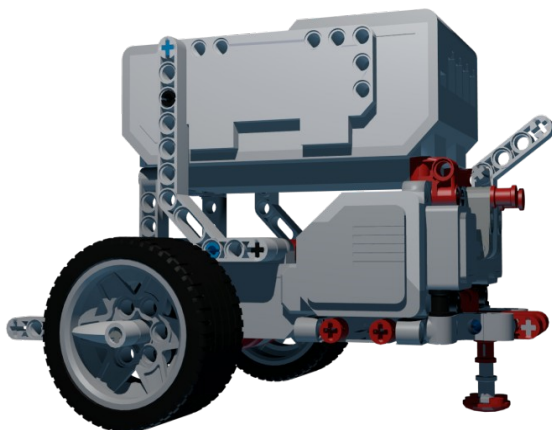
Two drive wheels and a skid. Manoeuvrable.
