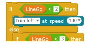
For sensors that output finer resolution numbers we might set the comparison number to "1.3" say rather than "2", but because our line Following Sensor outputs whole numbers we use the "<2" to pick up an output of "1".
