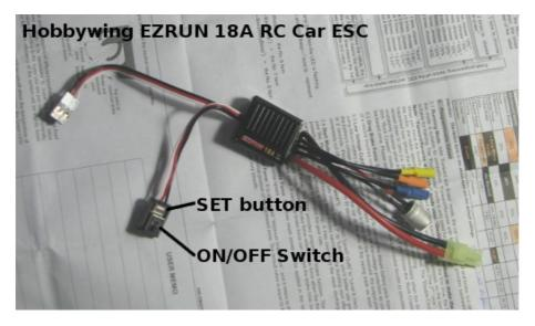
Programming and calibration of the **HobbyWing EZRUN 18A ESCs** was carried out without the ESCs being installed on the ROV electronics pod. Because the switch and "SET" button on the ESC are both accessible when the ESC is installed calibration and programming can be done at any time.
