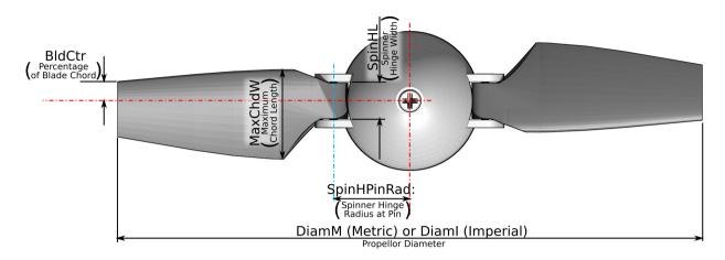
Here is a run down of the parameters used in the Folding prop model.
