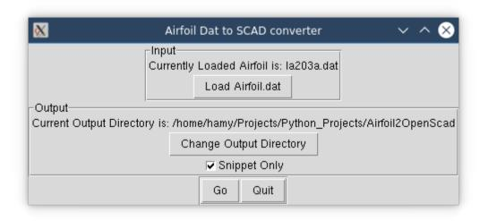
Once you have generated your OpenSCAD style version of the airfoil using this Python script, you can drop the Airfoil\_points list directly into these parametric propeller scripts in place of the existing Airfoil points list currently loaded with the NACA4412 airfoil.
