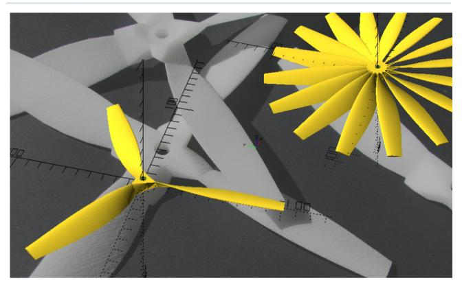
The script (currently) has the NACA4412 airfoil as the blade profile. This produces a very thin blade which is getting into the realm of being a bit too bendy. After a bit of testing I may replace this with a thicker airfoil. If you want to use a different airfoil look for the line;
