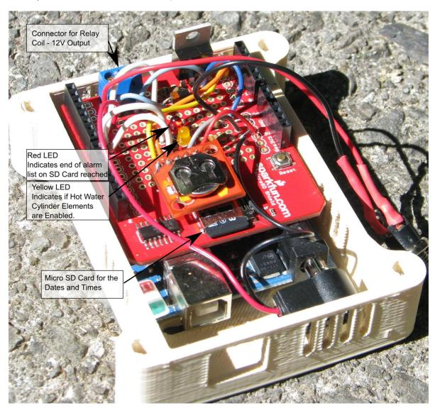
There are two Arduino sketches included on the SD card. One is for a NORMALLY CLOSED relay (*TimerDriverv3\_NC\_Variant*), the other is for a NORMALLY OPEN relay. Once set this should not need to be changed. There are programmes included on the SD Card to allow editing and reloading of the Arduino Sketch should that prove necessary.
