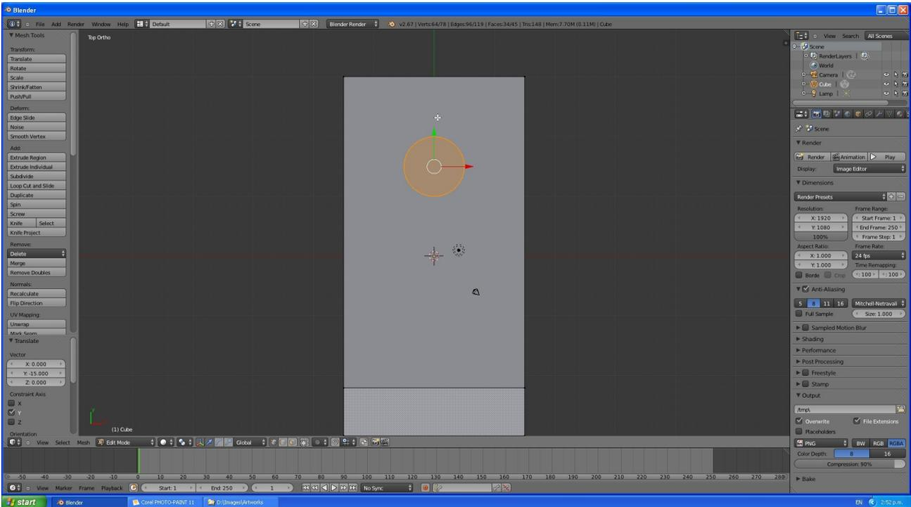
Move the cylinder to its position 15mm from the edge. ("gy-15 enter")
