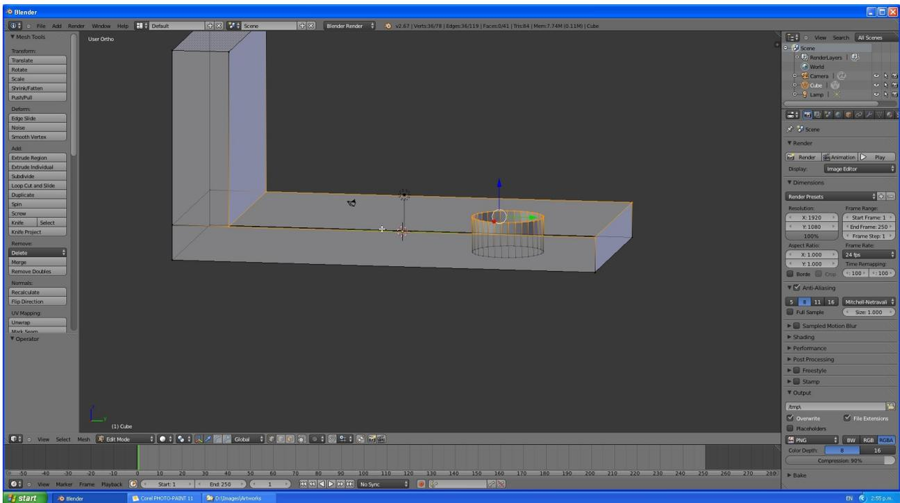
Yellow edges show that we have selected the top edge of the cylinder and the surrounding square of the bracket front face.
