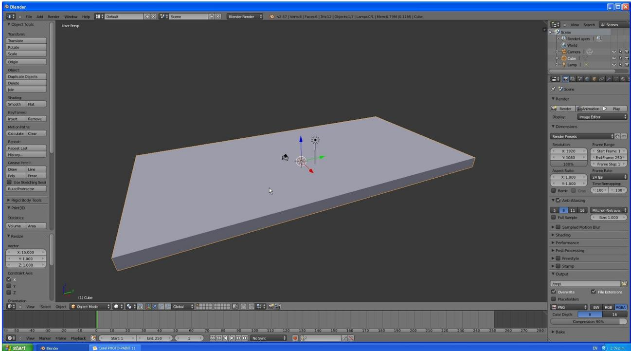
Scale the width to the width of the bracket. ("sx15 enter")
