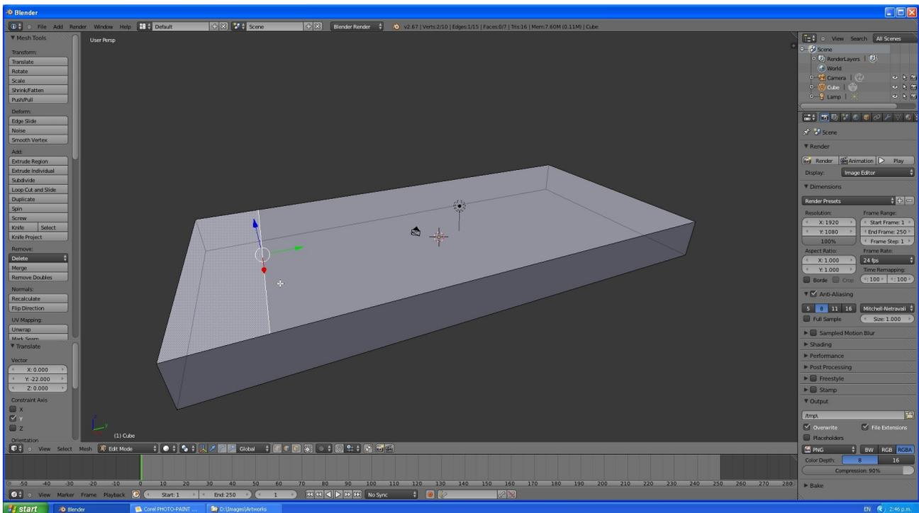
Drag it down to where it is 8 units from the end. In this case we know the edge occurred in the middle and so we can key in the exact measurements to move it  $30\text{mm} - 8\text{mm} = 22\text{mm}$  in the negative y-direction. ("gy-22 enter")
