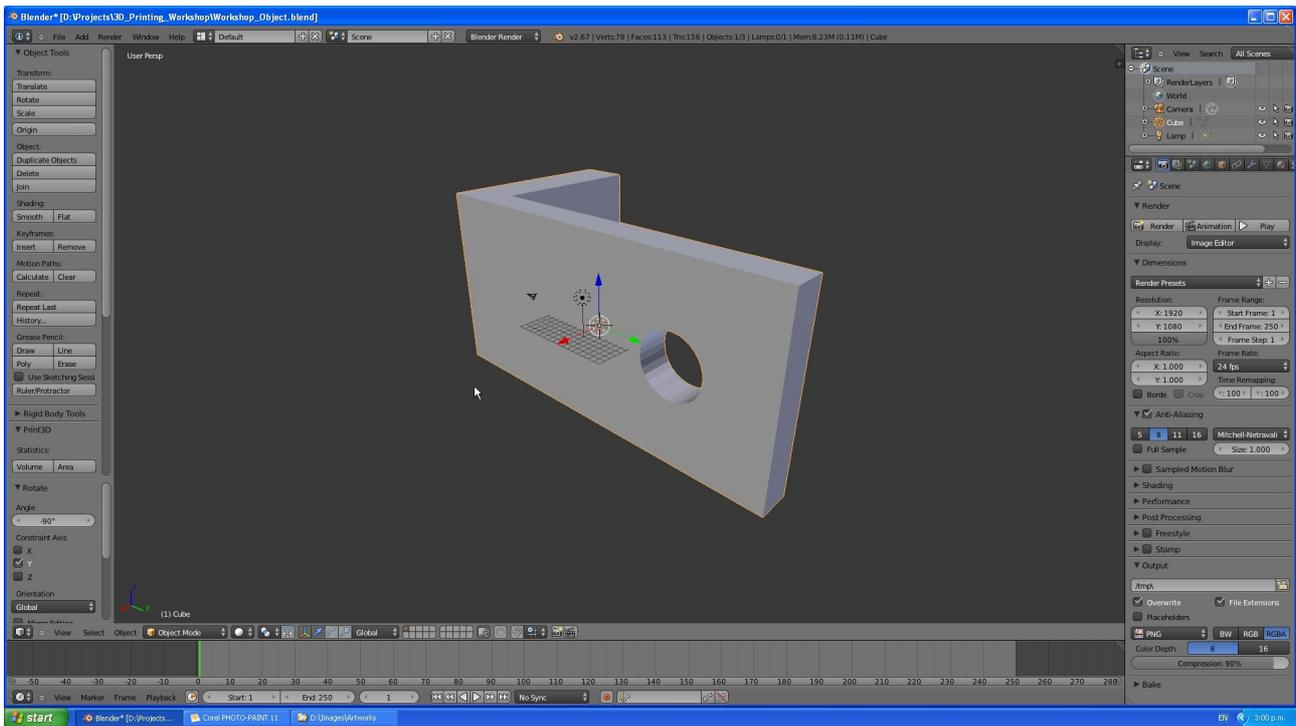
Rotate the object to an orientation that will be printable and maximise the strength.
