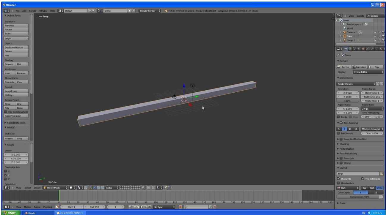
Scale the default 2mm x 2mm x 2mm cube out to the bracket length. ("sy30 enter")
