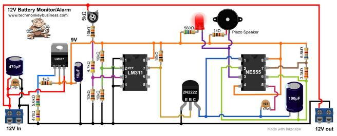
Here is the circuit laid out for a perf-board build.
